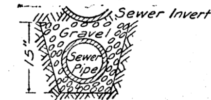
SEWER SUB DRAIN
