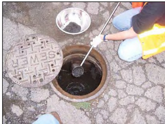
Figure 5: Inline grab sampling
