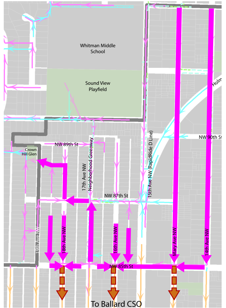
Figure 3.4.C Option C2: Partial reroute to Ballard Combined Sewer. Rerouting much of the upstream flow south through the Ballard CSO could help relieve the capacity and maintenance risks, but is only recommended if constrictions to the south have been fixed first. Also, portions of this option may require approval by and agreements with King County.
