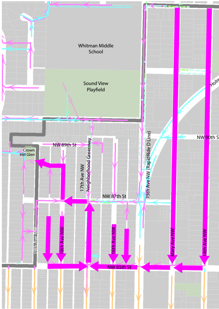
Figure 3.4.B Option C1: Maintain existing sewer flow. Capacity risk in this scenario could be reduced by fixing a downstream flow constriction to the northwest (see problem “C” in Figure 3.4.A). The portion through easements would continue to be a maintenance challenge.
