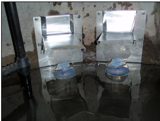
Figure 2.2.2.1d. Photo of R1 Sediment Traps
