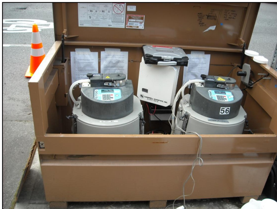
Figure 4.2.2.1f. Inlet Chamber showing Sample Tubing
