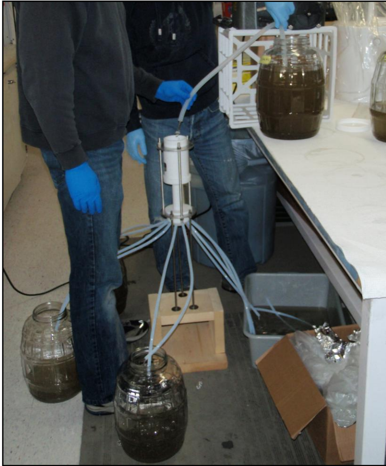
Figure 2.3.5b. Photo of Compositing Samples Using Cone Splitter
