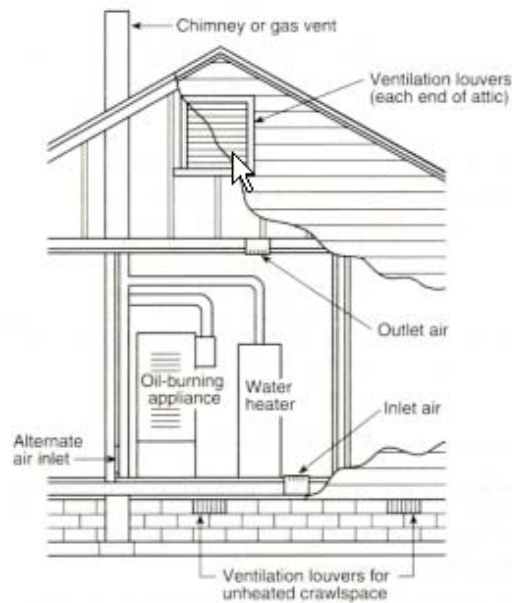
FIGURE 703.3.2(c) APPLIANCES LOCATED IN CONFINED SPACES— ALL AIR FROM OUTDOORS, WITH INLET AIR FROM VENTILATED CRAWL SPACE AND OUTLET AIR TO VENTILATED ATTIC
