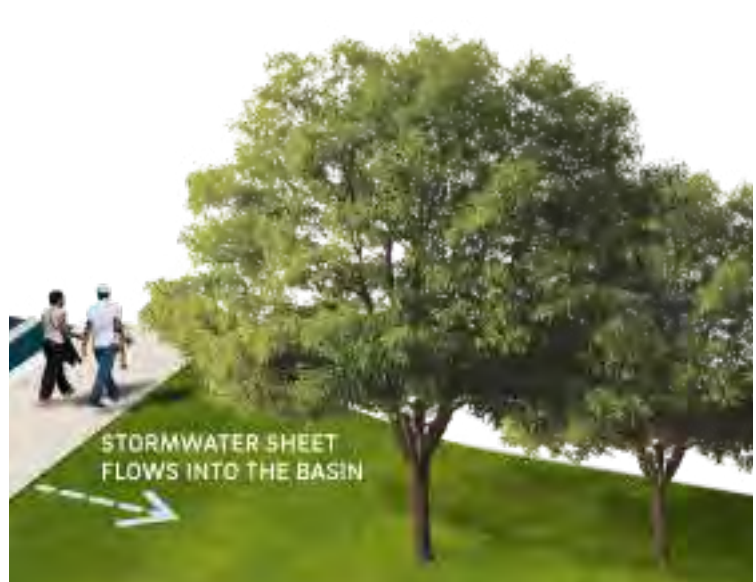
Stormwater dispersion into lawn and planting areas, reducing flow into the drainage system
