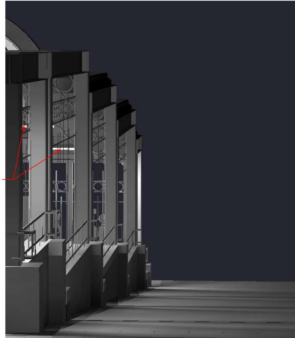
Pioneer Square Station (Prefontaine) Jefferson Street to 2nd Avenue 3D Rendering with Type LS2 light fixtures.
